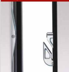
Two locking bolts generate the 15-mm, handle-driven closing and opening movement of the sash. Special polymer stops absorb the impact noise.
