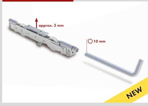
The height-adjustable bogie wheels make it possible to lift the rear sliding sash up to approx. 3 mm. This facilitates the quick and easy alignment of the sliding sash during assembly.
